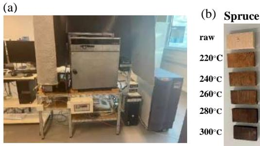
Fig. 1. (a) Photo of the torrefaction unit. (b) Chips collection from raw to highly torrefied
